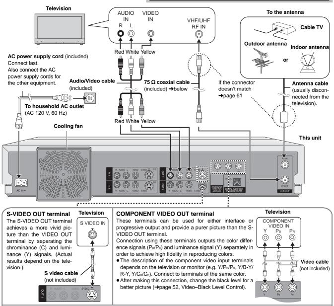
When making either of the above connections, ensure you connect the audio cables to the corresponding audio input terminals on the television.
